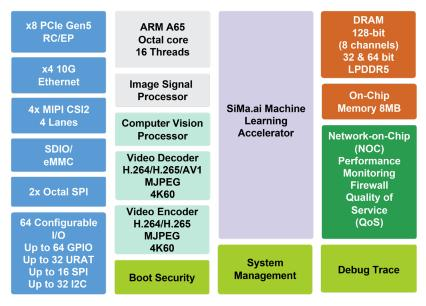
All architectural building blocks are seamlessly integrated via an internal, secure Network-on-Chip (NoC) architecture.
